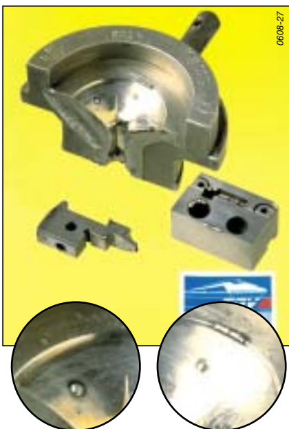
Repair and resurfacing of tools and moulds.
