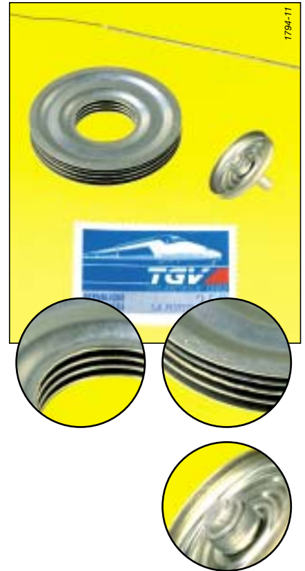
Welding membranes and thermocouple junctions.
