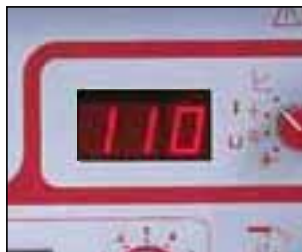
Short-Arc MIG, thickness < 3.0 mm.
