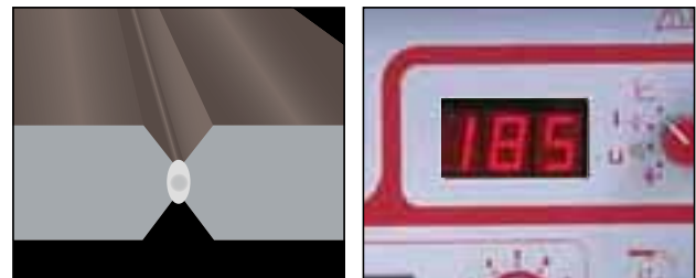
Penetration pass Short-Arc MIG, thickness < 25 mm.
